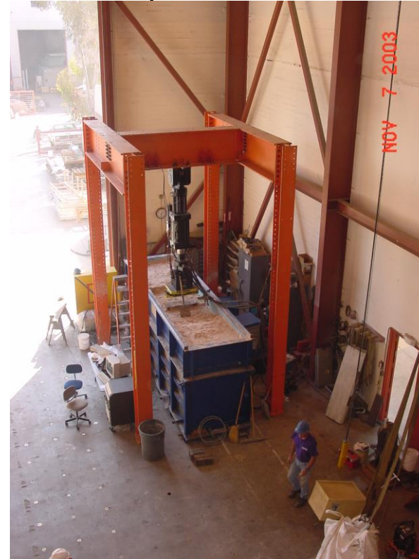
Rigid container for footing/pipeline testing with transparent acrylic side walls
