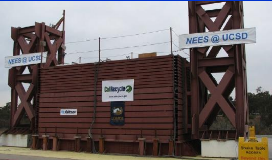
Laminar soil shear box: 6.7m (L) × 3.0m (W) × 4.7m (H)
