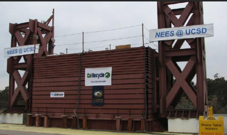
Laminar soil shear box: 6.7m (L) × 3.0m (W) × 4.7m (H)
