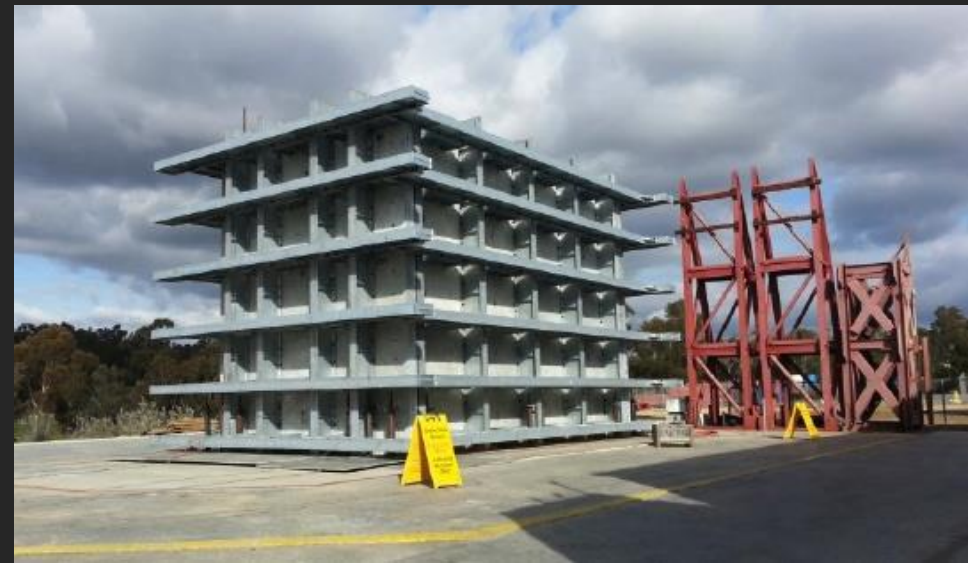
Stiff soil confinement box: 10.0m (L) × 4.6 or 5.8m (W) × 7.6m (H)
