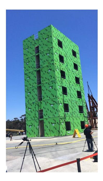
Earthquake and Post-Earthquake Fire Performance of Mid-Rise Light-Gauge Cold-Formed Steel Framed Buildings PI – Prof. Tara Hutchinson, UC San Diego
