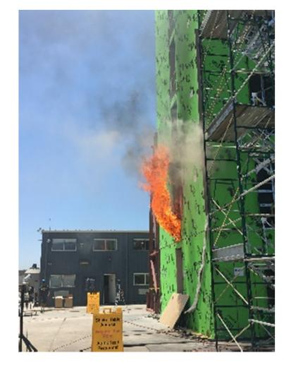
Earthquake and Post-Earthquake Fire Performance of Mid-Rise Light-Gauge Cold-Formed Steel Framed Buildings
