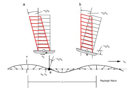
Geometric interpretation of how horizontal translation and rocking can contribute to the total drift in a simple building during passage of a Rayleigh wave [Trifunac, 2009]
