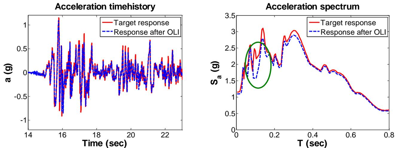
The target acceleration spectrum and the spectrum of the table motion did not match well for frequencies near 10 Hz.
