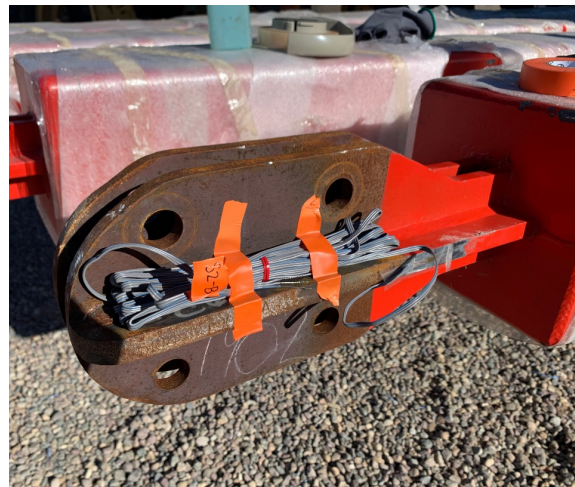
Strain Gages & LVDTs on BRB Core and Gusset Plates
