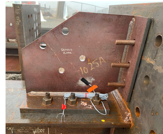
Strain Gages & LVDTs on BRB Core and Gusset Plates
