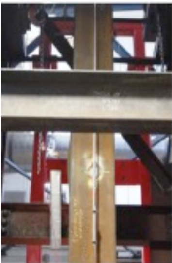
BRB Weak Axis Buckling
