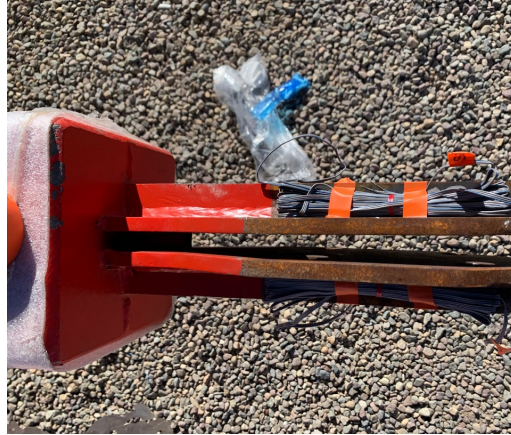
Strain Gages & LVDTs on BRB Core and Gusset Plates
