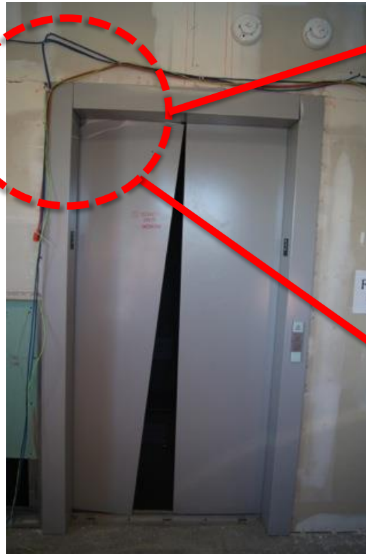
Door Jamb After FB6-DEN100 (non-functional)
