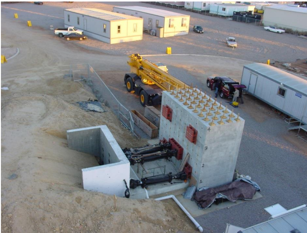
Bridge Abutment - Soil Interaction (Caltrans)
