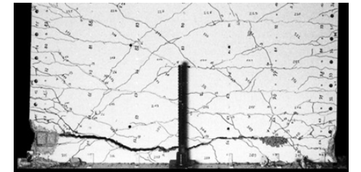
Tension failure ( Dazio et al. 2009)
