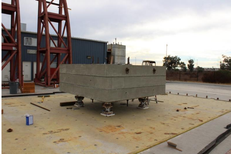
Figure 2: Experimental substructure for hybrid simulations
