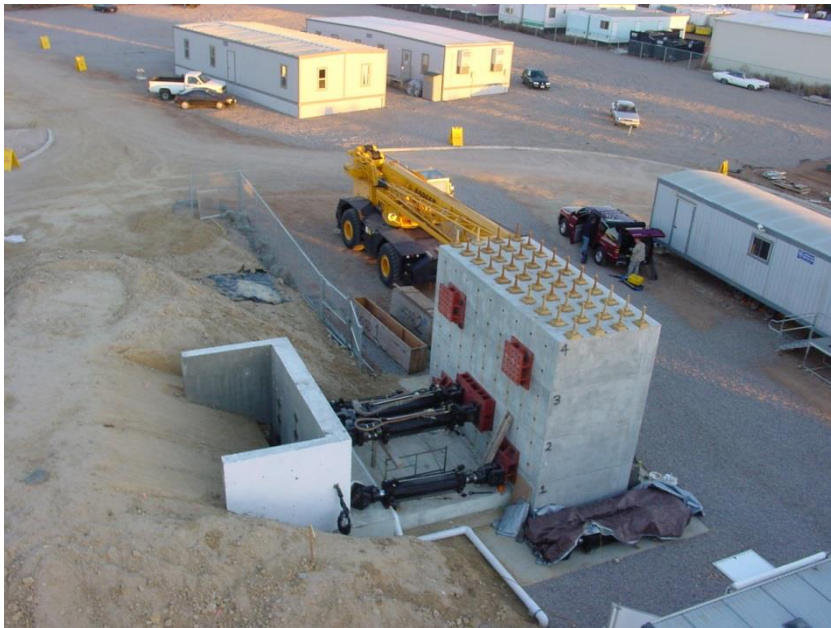
Bridge Abutment - Soil Interaction (Caltrans)
